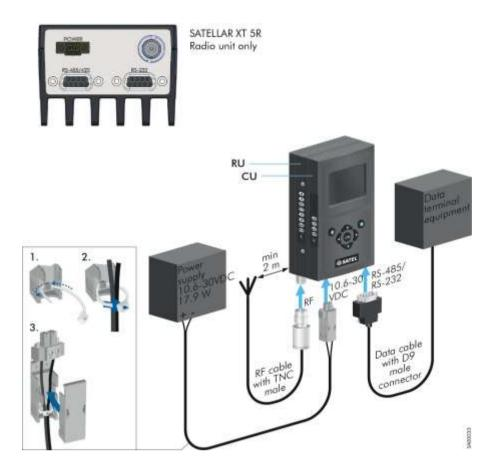
Figure 3.1 Transferring data through the RU, cabling
