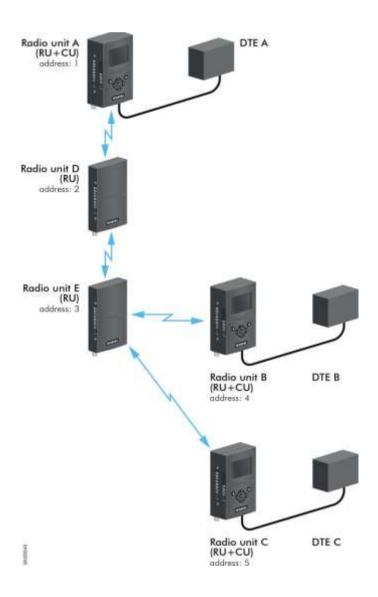
Figure 6.4 Routing example
