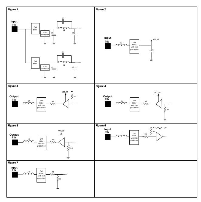
Figure 4.3 The module input-output equivalent circuits.
