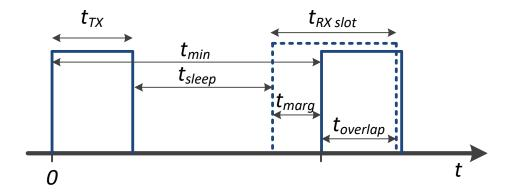
**Figure 7.1** Power save mode timing factors.
