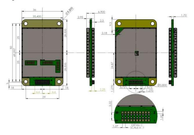
Figure 5.3 The module physical dimensions and the holes in millimeters.
