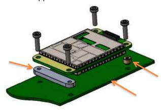
**Figure 5.1** Example of module attachment to application PCB.
