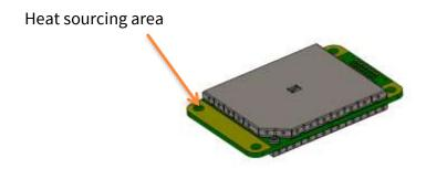
Figure 5.2 Heat sourcing area, both sides.
